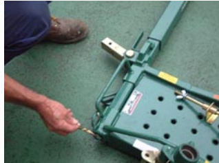
Fig 3 - Secure Wheel pan to axle shaft.
