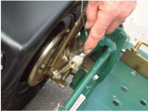
Fit Steering lock pin in this position when towing unladen.
