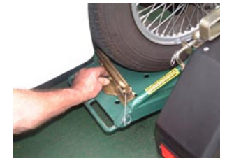
Fig 15 - Fit chocks to wheels.
