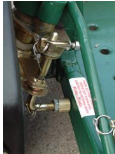
Fit Steering lock pin in this Position when reversing.
