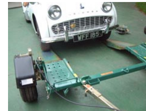
Fig 14 - Winch vehicle onto stowboy.
