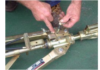
Fig 12 - Fit brake assembly to 'A' frame/hitch
