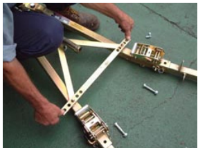
Fig 7 - Adjust 'A' frame and secure.
