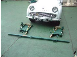
Fig 2- Line up wheel pans and axles (see Fig 2b).
