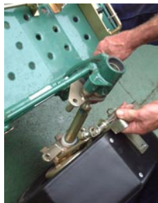
Fig 8 - Lift Wheel pan onto wheel stub.
