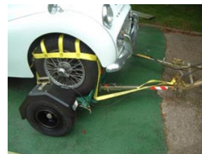
Fig 16 - Fit wheel nets to top of wheels.
