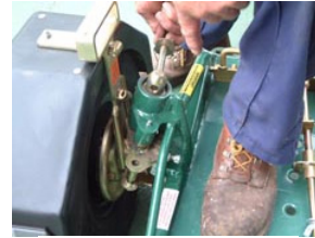
Fig 10 - Fit retaining pin to top of stub.
